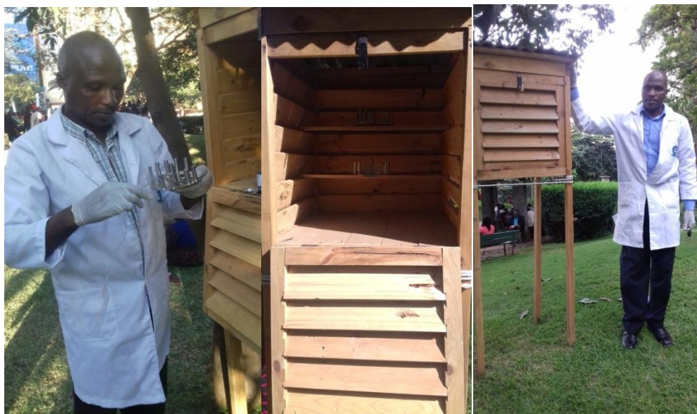
Plate 2: Photographs showing the deployment of SPMDs for air sampling
