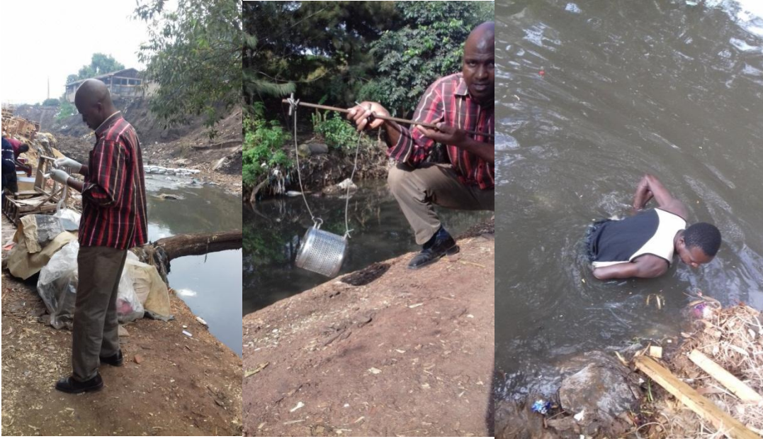
Plate 1: Photographs showing the deployment of SPMDs on surface waters
