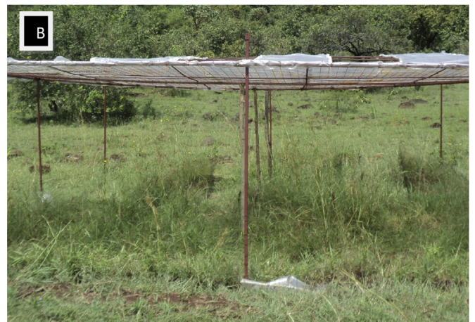
Fig. 1. (A) The layout of rainfall manipulation plots. Parallel arrows show transparent rainout gutters used to simulate rainfall reduction and direction to which excluded rainfall flows (rainfall increment plot/150% rainfall). (B) Photograph of rainfall manipulation plot with a slanting roof partially covered by transparent rainout gutters to exclude 50% of the rainfall and redirect it to the plot designated to receive more rainfall (i.e., 150% rainfall).
