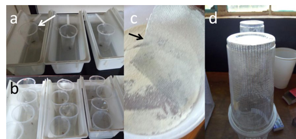
Fig. 1 Bioassay set-up. a Exposure of Anopheles gambiae larvae to one constrained Pantala flavescens in plastic cups (arrow) inside the larval bowl. b Exposure of An. gambiae larvae to four constrained P. flavescens kept in separate plastic cups. c Electrostatic net (arrow) treated by B. bassiana , used for exposing adult An. gambiae to fungus spores. d Exposure cup with the B. bassiana -treated electrostatic net inside
