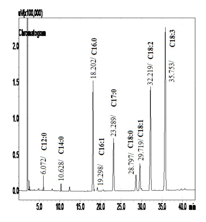
Figure 3: Chromatogram of a typical sample analyte
