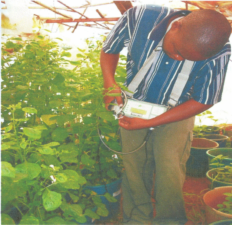
Plate 3.1 Measuring chlorophyll fluorescence and leaf temperature using a portable fluorescence monitoring system.
