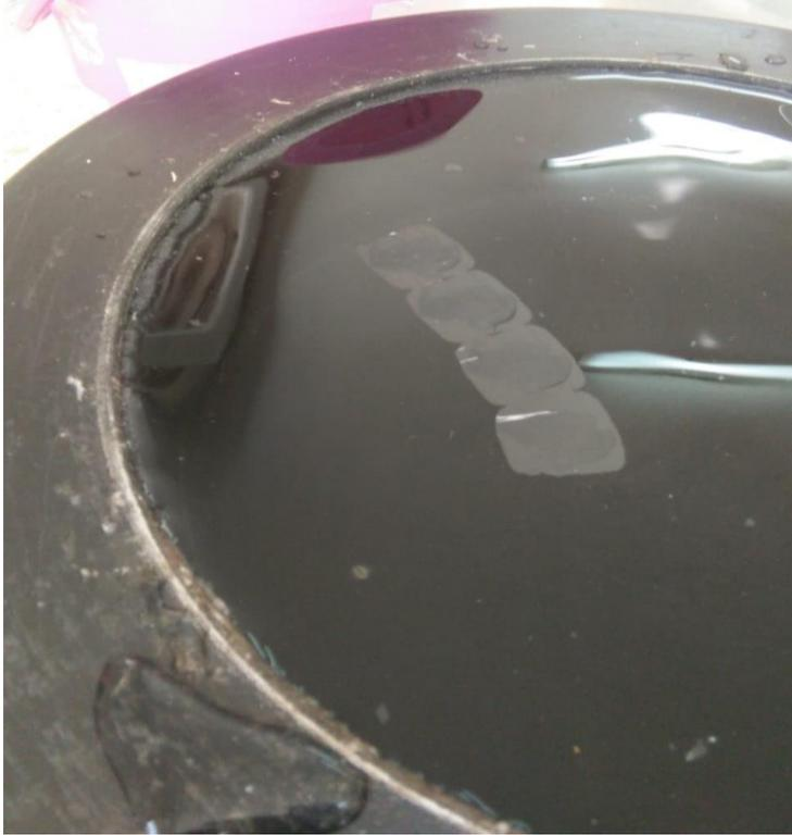
**Figure 5: Floating out water bath**
