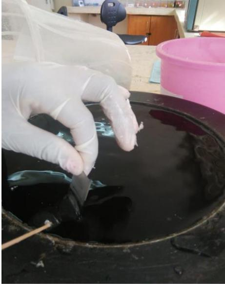
**Figure 6 : Fishing-out from a floating out water bath**
