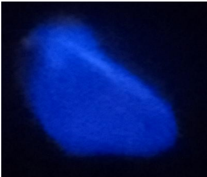
Figure 4.11: Flame produced on burning bio-ethanol
